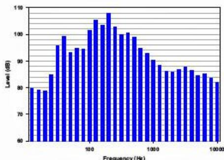
Fig 4 shows the noise spectrum for a stock car but in this case there is an additional noise frequency peak around 30Hz
