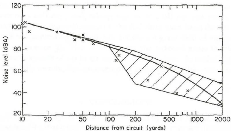
Fig 5 shows noise level measurements made at up to 800 yards from the track during car racing as a function of distance. No allowance has been made for wind or terrain differences but the hatched area in Fig 3 illustrates the divergence that occurs over 100 yards due to these effects.
