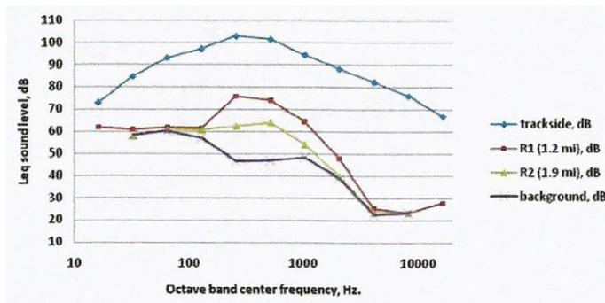
Fig 4. (fig3 ref24) A Stock Car noise Spectrum
