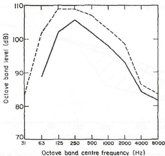
Fig 2 (Fig 4 Ref 6) shows the octave band average noise levels for both racing cars and motorcycles. There is in fact little variation and nearly all the important energy is in the 125, 250, 500 and 1000 Hz octave bands.
